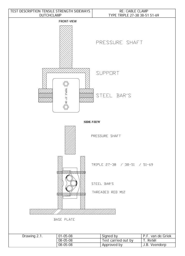
Test report tensile strength sideways cable clamp type TRIPLE 27-38 38-51 51-69.
