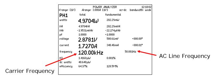
Phase 2 will also display the same two frequency components for the user's reference.
