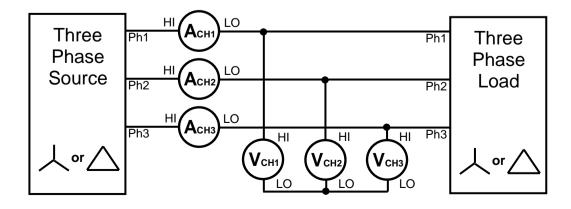
Three Phase Three Wattmeter – Star Connections
