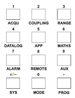
**SELECT MENUS** for non mode-specific configuration. Also use as numeric keypad when entering parameter values or data.
