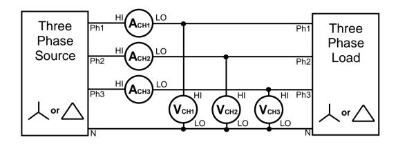
Three Phase Three Wattmeter – Delta Connections
